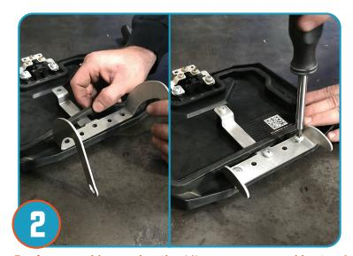
Replace new hinge using the (4) screws removed in step 1. Slide hinge between rubber gasket and glove box plastics.
