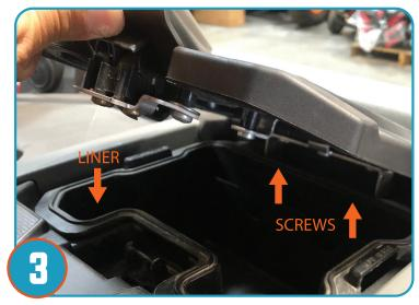
Re-insert the glove box liner then re-insert glove box lid with new hinge. The (2) screws removed in step 1 will not be re-used. Proceed with Pro Armor cage install.
