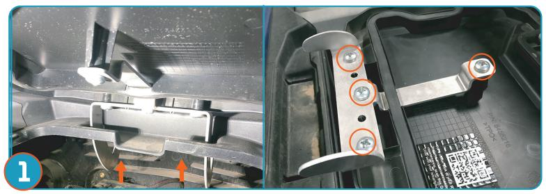
Remove glove box liner and remove (2) screws at the base of the hinge seperating it from the plastics. Remove (4) screws holding the hinge to glove box panel/lid.
